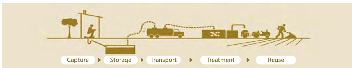
**Figure 3. Safely managed sanitation system providing protection from exposure to hazards across the sanitation service chain** (Source: Rohilla et al., 2017)
