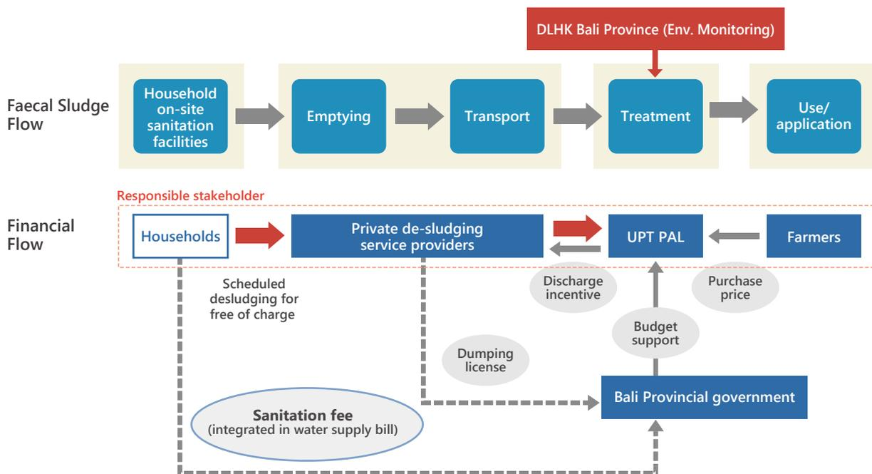
Figure 8. Example of incentivized discharge model proposed for faecal sludge emptying, collection and transport, treatment and reuse in Denpasar city of Indonesia (Bao, 2019b)
