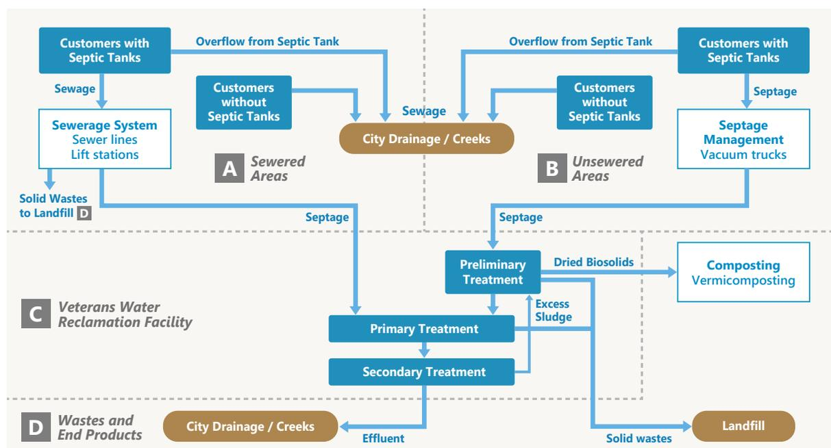
Figure 4. Selection of appropriate technology at Veterans Water Reclamation Facility (The Philippines) for combined sewage and faecal sludge treatment. (With daily treatment capacity: 2,400 m<sup>3</sup> of sewage, 240 m<sup>3</sup> of faecal sludge)
