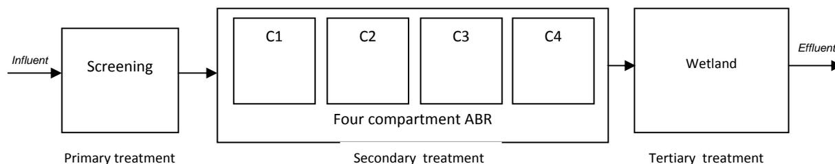
Figure 2. Scheme of ABR and wetland system for treating small scale yarn dyeing waste water.
