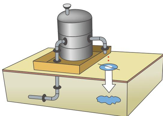
**Figure 2.4.9** Underground infiltration of hazardous substances from production facilities (Source: provided by MoEI)
